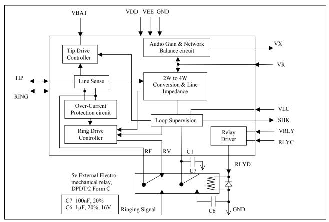
Figure 1 - Dual Channel SLIC Single Channel Schematic Diagram
